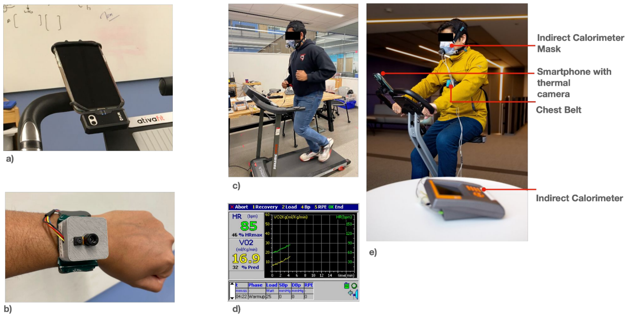
Fig 2: JoulesEye's is composed of a thermal camera retrofitted in an iPhone as shown in (a). JoulesEye can be used in a smartwatch as shown in b). The camera in b) is a low resolution (32x24) thermal camera. (c) and (e) show the ground truth data collection procedure with indirect calorimeter while running and biking. (d) shows a screen grab from the indirect calorimeter recording the energy expenditure during an exercise session.
